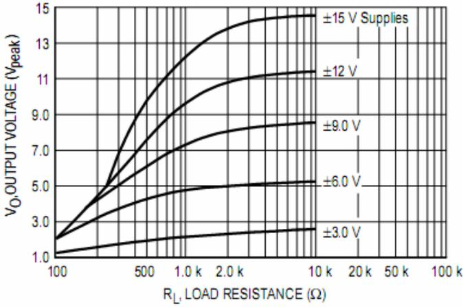
Figure 9. Negative Output Voltage Swing versus Load Resistance
