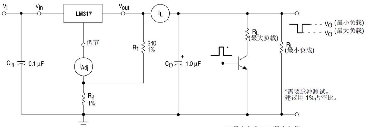
负载调整率(mV)= $V_O(\text{最小负载})-V_O(\text{最大负载})$
